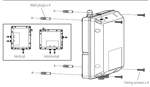
**Warning!** Please check for any hidden cables and pipes before drilling holes in the wall.
